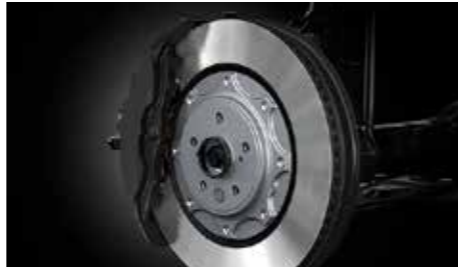
Opposed 6-piston brake caliper (front)
