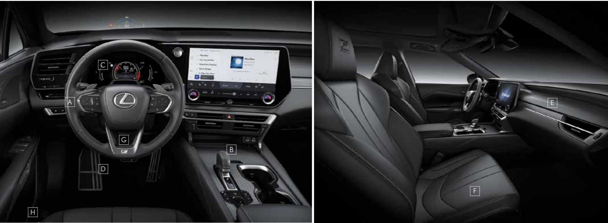
F SPORT Performance/F SPORT features A_Dimpled leather steering wheel with paddle shifters / B_Dimpled leather shift knob / C_TFT meter / D_Aluminum sport pedals and footrest / E_Real aluminum ornamentation / F_Leather sport seats F SPORT exclusive features G_Emblem / H_Scuff plate
